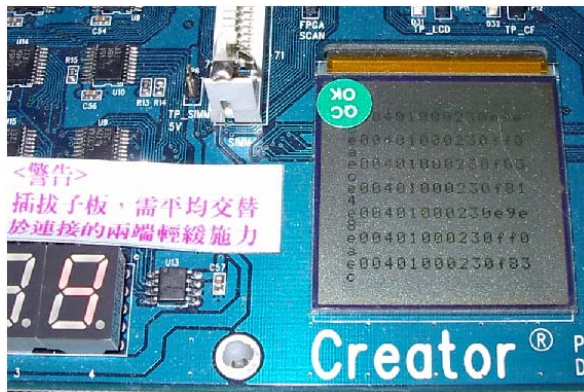
Figure 14. Display Interface of Embedded System in Executing Mode.
