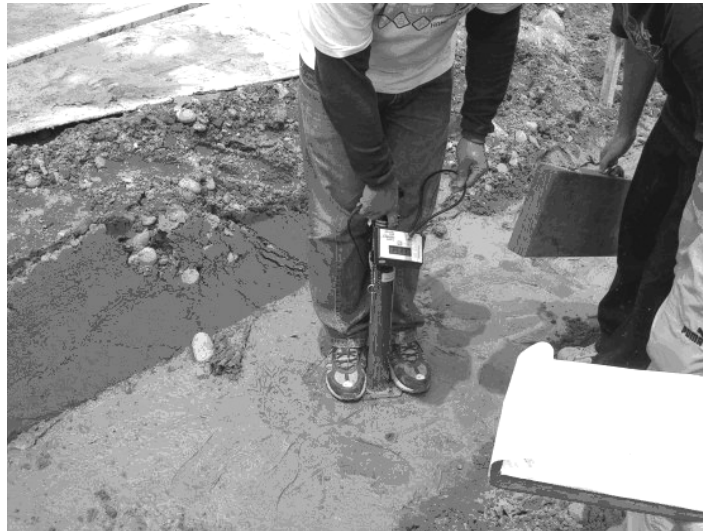
Figure 9. Examine the bearing capacity with Clegg Impact Tester
