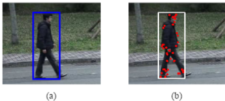
Fig. 3 (a) Example of blob-based object detection, (b) SURF feature points (red dots) are located in the object region.
