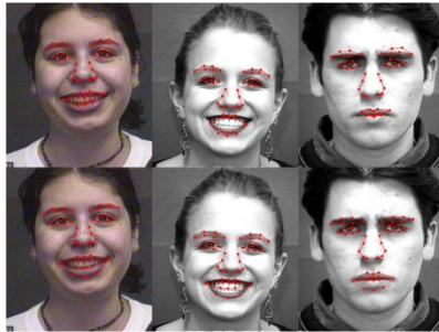
Fig. 10. Some results on the Cohn Kanade database. The top row shows the detected landmarks by the traditional ASM method and the bottom row shows the detected results by the proposed ASM method.
