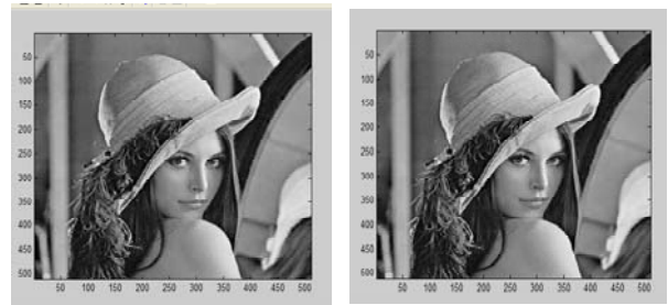
(a) (b) Fig. 12 512 x 512 Lena (a) Original image (b) Reconstructed image (9/7 DWT with 4-level)
