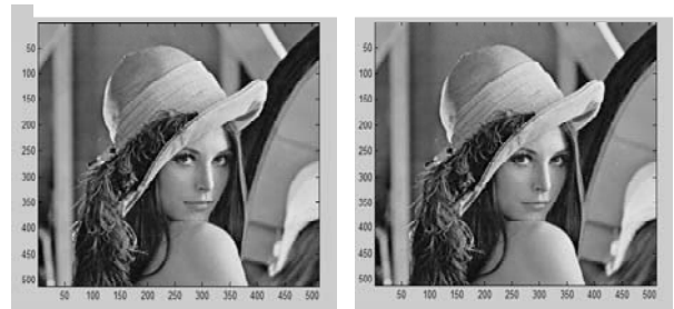
(a) (b) Fig. 13 512 x 512 Lena (a) Original image (b) Reconstructed image (5/3 DWT with 4-level)
